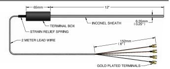
It can be manufactured to any length using the following part numbers:
