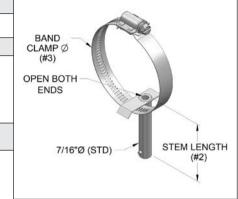
**Note:** L = Length of stem. Should be equal to the maximum insulation thickness + 3/4". The bayonet sensor length for adjustable should be L + 1-1/4". For fixed, it should be L + 1/2".
